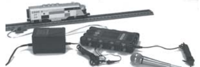
External Microphone Attaches To TIU Proto-Dispatch Port
