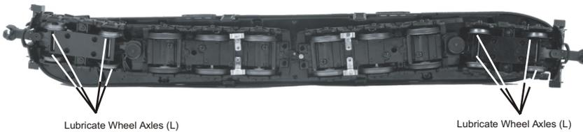
Figure 1. Lubrication Points on the Locomotive
