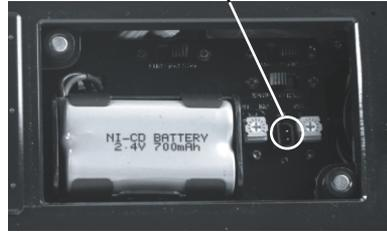
Figure 9. Battery Charger Port location.
