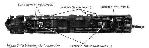
The locomotive's internal gearing was greased at the factory and should not need additional grease until after 50 hours of operation or one year, whichever comes first.
